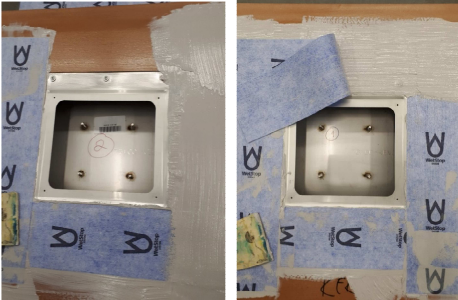
Picture 1-2. Preparation of test specimens WetStop KL-tape.
